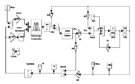
Fig. 9.31. Fuzzy logic controller model
