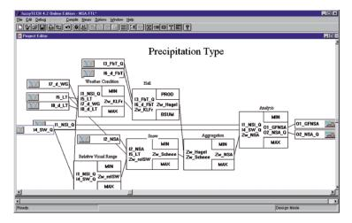
Fig. 8.46. Precipitation type fuzzy logic module
