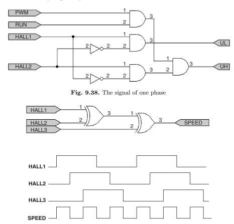
Fig. 9.39. The speed pulse multiplexer
