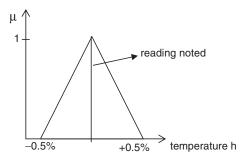
Fig. 4.5. Membership functions representing imprecision in crisp temperature reading
