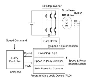
Fig. 9.37. Overall system block diagram
