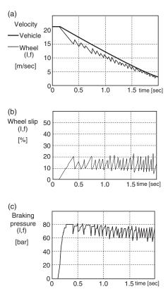
Fig. 8.89. Simulations of a full braking
