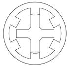
Fig. 9.1. SRM with six poles on the stator and four poles on the rotor
