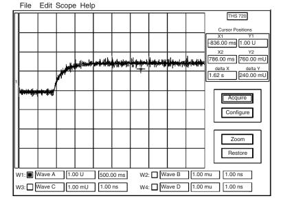
Fig. 9.48. The unit step response to no load
