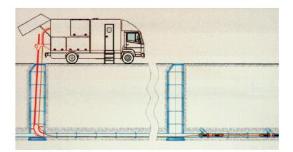
Fig. 8.65. The two robot units in the sewage pipe (right) are supplied from a specialized truck by cables
