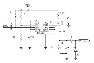
Fig. 9.46. The circuit of  $\mathrm{F}/\mathrm{V}$  converter
