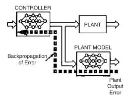
Fig. 8.114. Error propagation through plant model
