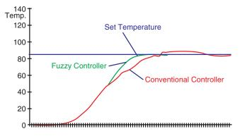
Fig. 8.68. The fuzzy logic controller in the molding machine reaches the set point faster and avoids overshoot
