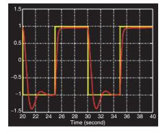
Fig. 9.26. Closed-loop response with the gain-scheduling fuzzy controller
