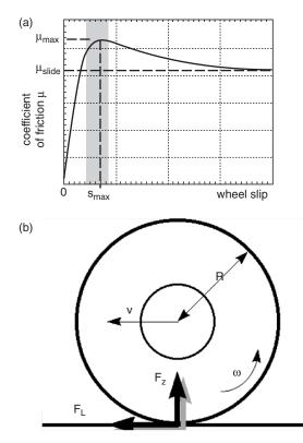
**Fig. 8.80.** (a) Friction characteristics; (b) Wheel model  $F_z$ : Wheel load; R: Wheel radius;  $\omega$ : Angular wheel frequency; v: Velocity of wheel center;  $F_L$ : Longitudinal force
