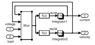
Fig. 9.8. Linear model of DC motor
