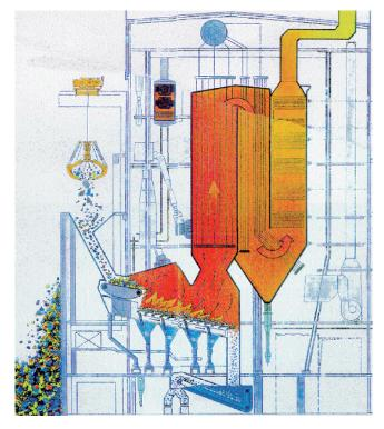
Fig. 8.62. In a waste incineration plant, a crane continuously delivers waste from the bunker to the belt running through the burning zone. The exhaust gases are cooled and cleaned
