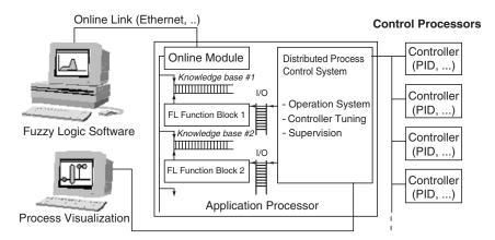
Fig. 8.52. Integration of a fuzzy logic component in a distributed control system
