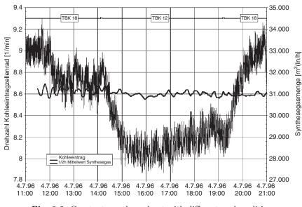
Fig. 8.9. Constant gas throughput with different coal qualities
