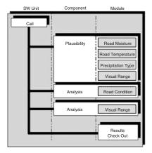
Fig. 8.43. Architecture of environmental data analysis
