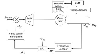
Fig. 8.129. Modeling of load frequency control
