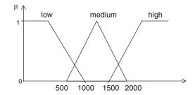
Fig. 4.6. Membership for fuzzy variable "speed" in rpm
