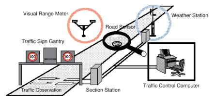
Fig. 8.42. Environmental and traffic sensors in a traffic control system
