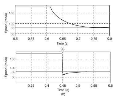
Fig. 9.6. Speed change from 180 to  $80 \text{ rad s}^{-1}$ : (a) without feeding and (b) feeding the phase with decreasing inductance
