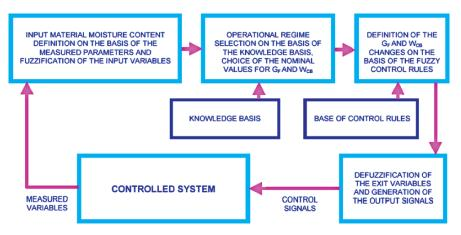
Fig. 8.95. Structure of the fuzzy control system for direct rotary dryer
