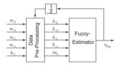
Fig. 8.82. Estimation of car velocity
