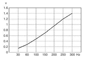
Fig. 9.47. The frequency response of  $\mathrm{F}/\mathrm{V}$  converter
