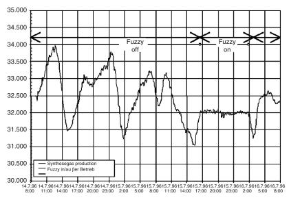
Fig. 8.6. Throughput control with and without fuzzy control
