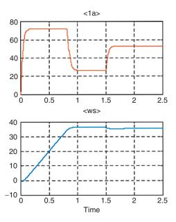
**Fig. 9.10.** Current (*upper red*) and angular velocity (*lower blue*) of DC motor. Simulink and linear model were used for simulation
