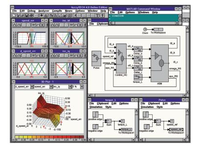
**Fig. 8.32.** Simulation of the enhanced fuzzy flux controller using the software products *fuzzy*TECH and Matlab/Simulink
