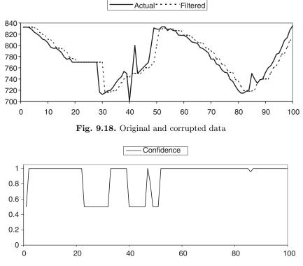
Fig. 9.19. Confidence of corrupted sensor signal
