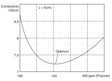
Fig. 8.54. Thick slurry conductivity over polymer proportion
