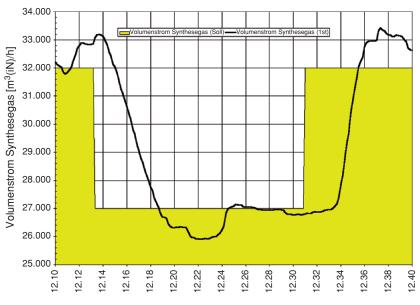
Fig. 8.7. Change of load with fuzzy control
