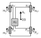
**Fig. 8.81.** Sensors and actuators of the experimental car CG: Center of gravitiy;  $a_x$ : Longitudinal acceleration;  $w_{i,j}$ : Angular wheel frequency; HU: Hydraulic Unit;  $p_{i,j}$ : Wheel brake pressure; *i*: l=left, r=right; *j*: f=front, r=rear
