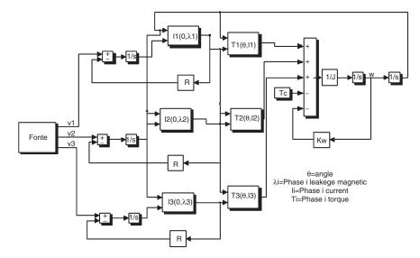
Fig. 9.2. Block diagram of the simulation
