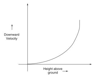
Fig. 8.121. Landing approach of an aircraft
