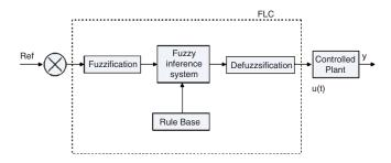
Fig. 8.130. Block diagram of fuzzy logic controller
