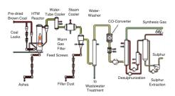
Fig. 8.2. Process diagram of HTW plant
