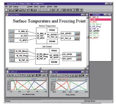
Fig. 8.45. Road temperature fuzzy logic module
