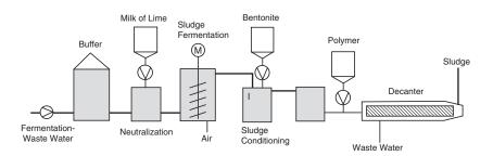
Fig. 8.53. Process diagram of sludge draining
