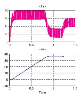
**Fig. 9.11.** Simulated current signal (*red*) and angular velocity (*blue*) using Simulink and Power System Blockset (PSB)
