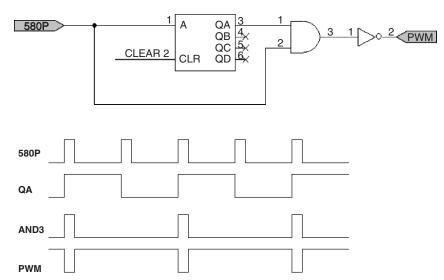
Fig. 9.40. The PWM resolution converter
