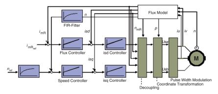
Fig. 8.29. Field-oriented control of AC induction motors
