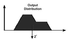
Fig. 6.3. Defuzzification using the center of mass
