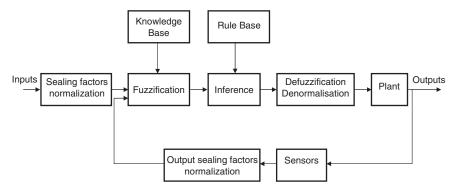
Fig. 8.120. Simple fuzzy logic controller
