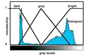
Fig. 8.14. Histogram fuzzification with three membership functions
