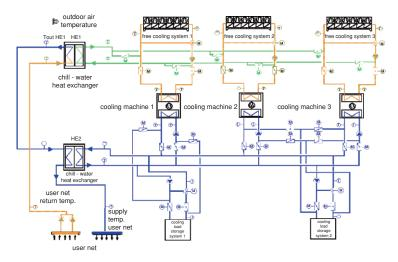
Fig. 8.74. Schematic diagram as a part of the chilling system with simplified instrumentation
