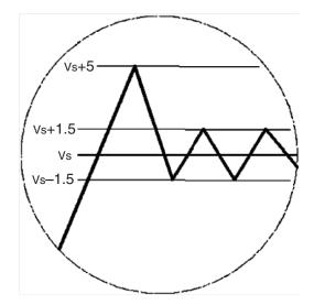
Fig. 8.34. Tolerances for the operation of the speed limiter
