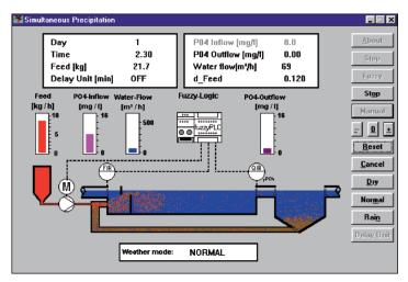
Fig. 8.64. A software simulation of a simplified precipitation controller
